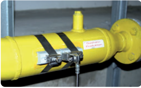
Pipe clamp for safe electrical contacting of pipes in Ex areas for implementation of lightning equipotential bonding according to IEC 62305-3 EN 62305 (VDE 0185-305-3)
